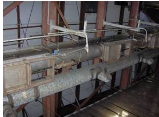
Figure 0-3 - Rotary Dewatering Presses and Sludge Conveyor
