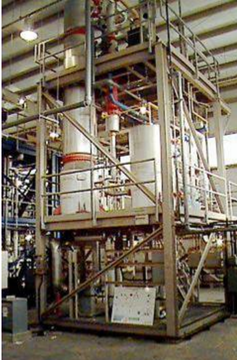
Figure 0-6 - Steam Stripping System Schematic
